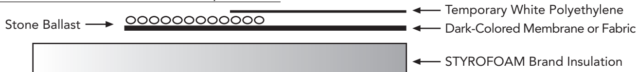
Sketch A: Dark-Colored Membrane, Ballasted
